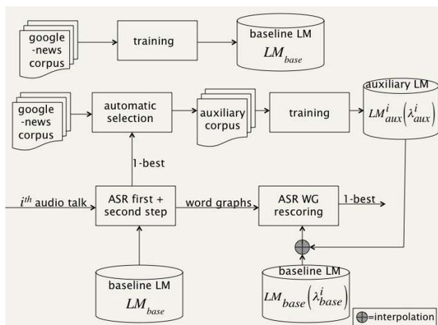
Figure 1: Block diagram of the ASR system.
