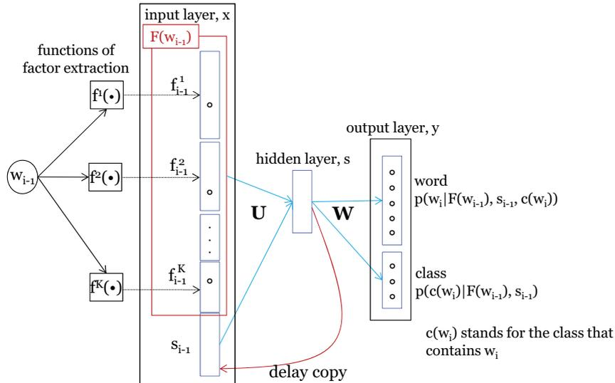
Figure 1: Architecture of factored recurrent NNLM.
